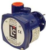
**Pulse output device**—Weights and Measures approved, provides a high resolution, unscaled pulse stream. The meter rotor is magnetically coupled to an optical encoder that has a signal which is directly proportional to the liquid flow through the meter. No dynamic seals to fail or leak. Easily adapts to most remote totalizers, batch controllers, computers, and other scalable pulse receiving devices.
