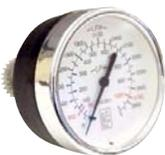
**Mechanical rate-of-flow indicator**—Direct-reading dial providing instantaneous response and dependable accuracy to within 1% of flow rate through meter. Cast aluminum case with ball bearings throughout. Readouts available in gallons, liters, and dekaliters per minute.
