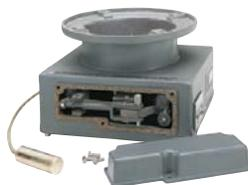
**Mechanical temperature volume compensator**—Uses a fluid-filled capillary system to sense product temperature and automatically correct counter reading for product volume changes due to temperature. When the temperature is 60° F, a 1:1 output ratio is supplied to the register. Output ratio is adjusted upward or downward depending on temperature fluctuation around 60° F.
