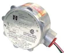
**Counter-mounted pulser**—Supplies an electrical signal to remote totalizers, batch controllers, rate-of-flow recorders, etc. Pulser models include dry reed (1 or 10 pulses per revolution), solid state single channel (100 pulses per channel) or solid state quadrature (50 pulses per channel).
