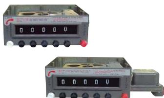
**Mechanical preset counter**—Available for either single-stage or two-stage valve closure. Sets a predetermined volume and controls a mechanically linked valve. Optional microswitches convert mechanical motion to an electronic signal for control of remotely located valve, pump, and alarms.
