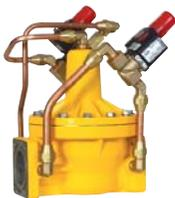
**Valve**—Diaphragm type, electrically (solenoid) actuated, aluminum body available with flanged or NPT connections. All valves provide downstream to upstream thermal relief and fail-safe closure. Provides presetting capability when used with electronic registers, such as LectroCount.
