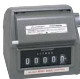
**Mechanical counter with ticket printer**—Large-numeral counter provides 5-digit resettable and 8-digit non-resettable totalizers. Printer generates an imprinted record of the transaction which is legal for use in resale applications.
